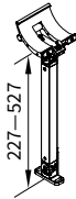
raised cassette bracket foot can be tilted backwards by up to 45°, head of cassette fixture bracket can be tilted forwards by up to 45°
